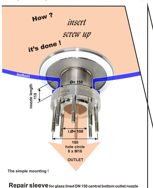
Is an enameled bottom outlet nozzle size DN 150 damaged on the inside neck or flange face, it can be repaired by the EC repair sleeve. The sleeve is made of steel and covered with solid PTFE. The mounting is simple, insert the sleeve from inside and screw it up from outside - no drilling and welding work is necessary. The new bottom outlet has the size DN 100.
